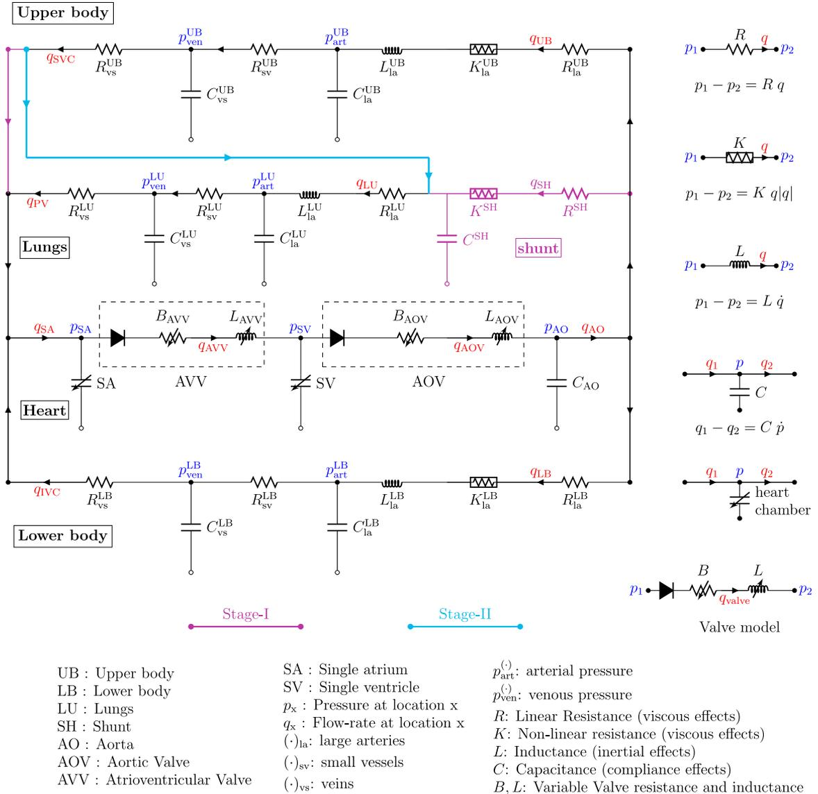
Fig. 1. Lumped parameter model for Stage 1 and Stage 2 single-ventricle physiology; pressures at major locations are represented in blue and flow-rates in red (see key for details).
