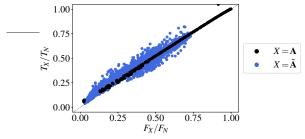
Fig. 5: Normalized number of flops vs. normalized running times for ISTA ( $tol=10^{-5}, \, \Gamma=0.5$ ). Each point on the graph corresponds to an independent run at a given regularization  $\lambda/\lambda_{\rm max} \in [10^{-2},1]$ . Results for the usual GAP Safe test are shown in black and those using its stable version (as in Alg. 1) are shown in blue. The closer the dots lie to the identity line, the better the theoretical speedups are met in practice.
