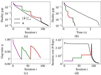
Fig. 3: Application example of the proposed algorithm. (a) and (b) Duality gap over the iterations and time respectively. (c) Gap ratio  $\gamma_t$  (cf. (29)) for the convergence switching criterion, with threshold  $\Gamma=0.2$ . (d) Computational complexity per iteration (worst-case theoretical number of flops, cf. section IV-B). N=2500, K=10000,  $\lambda/\lambda_{max}=0.2$ .
