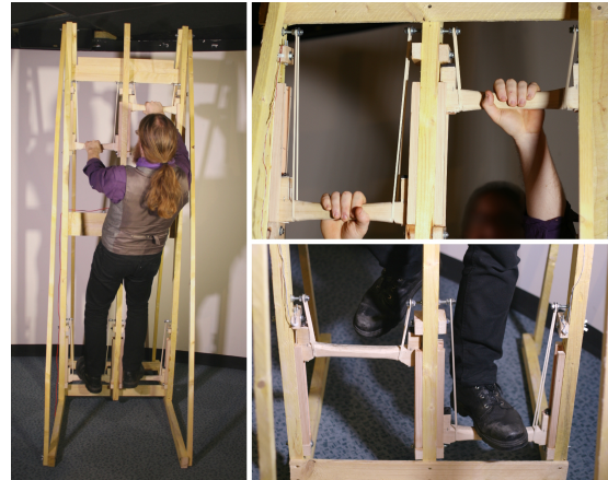
Figure 1: Left, the VladdeR , a tangible interface for Virtual ladder climbing. Right-up, the hands rungs. Right-down, the feet rungs.
