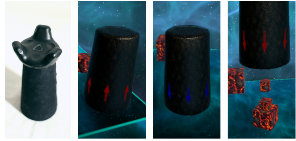
Figure 3: Illustration of the Dice Cup metaphor. From left to right, tracked tangible cup, grab operation, release confirmation after shaking the cup and lift of the cup revealing the stacked objects.
