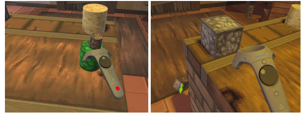
Figure 3: Physical object manipulation (left) with frame recording as indicated by the red round on the controller and time control (right), the green arrow indicates the object velocity, the pad can be rotated to navigate in the time-line as shown by the blue slider on the controller
