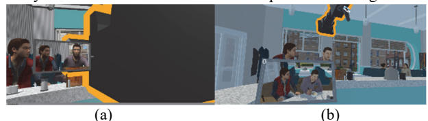
Figure 3: Emulating virtual camera through a 3D camera model and detachable panel screen. (a) attached (b) detached
