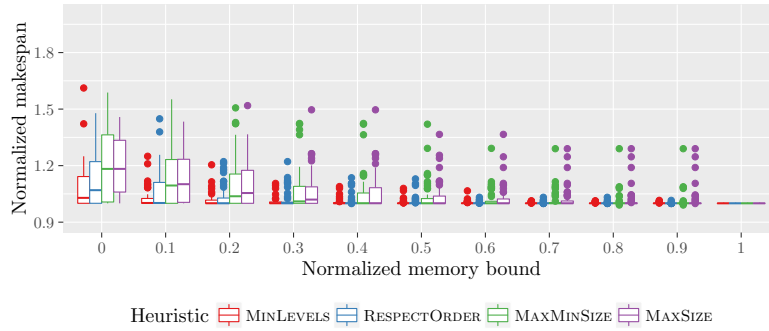
Figure 7: Makespan obtained by each method for the sparse DAGGEN dataset. The makespan plotted is divided by the original makespan. A memory bound value of 0 corresponds to the memory used by a DFS schedule, and a memory bound value of 1 corresponds to the maximum peak memory of the original graph.
