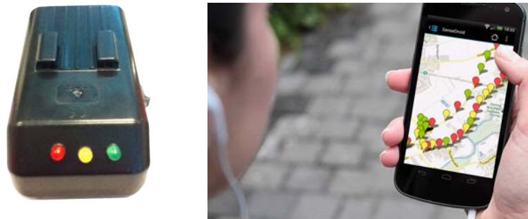
Fig. 7: NoxDroid situated analytics. Left: sensor with embedded pollution indicators. Right: smartphone application with contextual measures.
