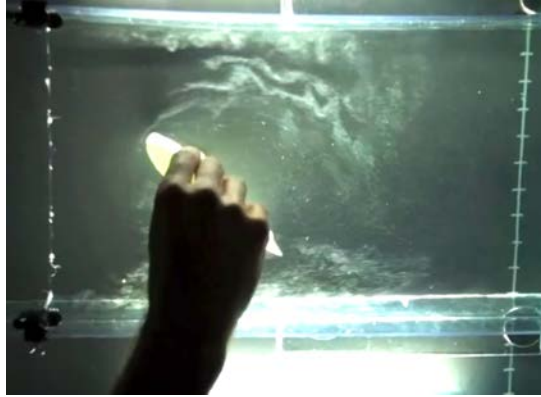
Fig. 6: A water tunnel visualization where a wing model can be rotated to examine the impact of orientation on aerodynamics [32]. Here the physical referent is the wing and the physical presentation is the set of water bubbles.
