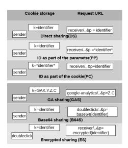
**Fig. 2.** Detecting identifier sharing. "Sender" is the domain that owns the cookie and triggers the request, "receiver" is the domain that receives this request and "identifier" is a cookie value that we detected as *identifier cookie*. "\*" represents any string.
