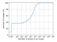
Fig. 1. Cumulative function of the number of pixels in images with a content-length less than  $100~\mathrm{KB}$ . 35.66% of images are invisible pixels: 9.00% have no content (they are shown as zero-pixel images) and 26.66% are of size 1x1 pixels.
