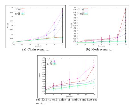
Fig. 6 End-to-end delay for the three scenarios.
