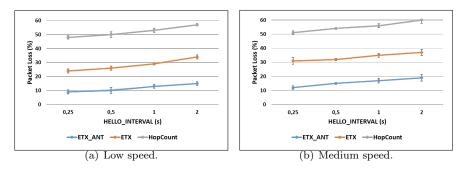
Fig. 10 Packet losses for different HELLO\_INTERVAL and two speeds. TC\_INTERVAL=5 sec.
