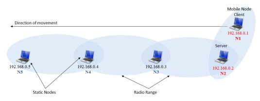
Fig. 8 Chain and wireless links in the testbed.
