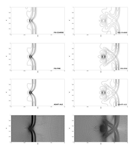
Figure 10: Small perturbation of a lake at rest (RD scheme). Solution isolines at t=0.24, t=0.48 are shown for fixed grid and adaptive computations. Top: fixed coarse grid. Middle: fixed fine grid. Bottom: adaptive ALE scheme.
