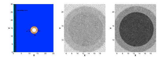
Figure 15: Conical island. Left: sketch of the computational domain with gauges. Middle: static coarse mesh topology. Right: static fine mesh topology.
