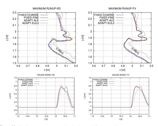
Figure 22: Okushiri experiment computed with adaptive ALE schemes. Top row: maximum runup for RD (left) and FV (right). Bottom row: total water height  $\eta$  signal registered at the gauge placed in the Monai valley. RD (left) and FV (right).
