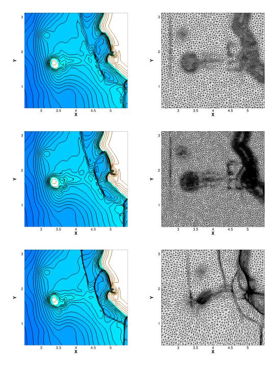
Figure 20: Okushiri experiment. Contour lines for h and mesh at  $t=16.5\,[s]$ . Top: fixed coarse grid. Middle: fixed fine grid. Bottom: adaptive ALE scheme.
