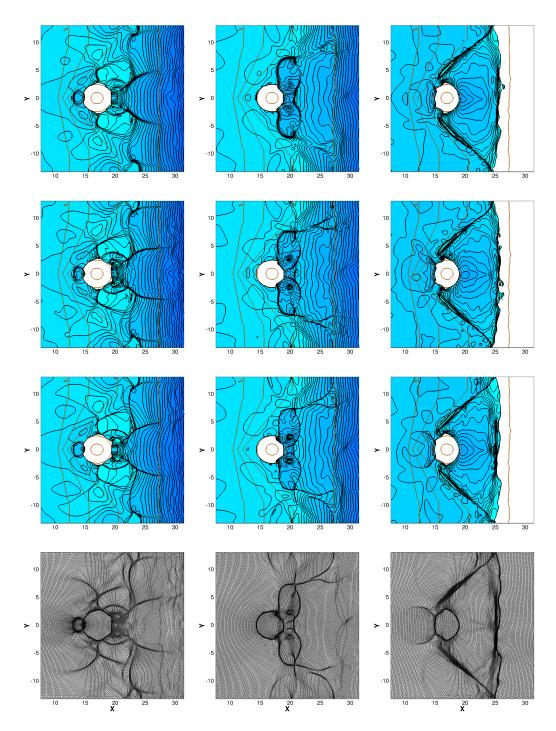
Figure 25: Solitary wave on a shelf (RD scheme). Solution isolines at t=0.24, t=0.48 are shown for fixed grid and adaptive computations. First row: fixed coarse grid. Second row: fixed fine grid. Third and fourth: adaptive ALE scheme.
