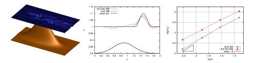
Figure 2: Linear Advection. Left: Lake at rest for the NO WB ALE formulation and failing in verifiying Well Balanced. Middle: comparison between the numerical solution and exact one on the simmetry line x=0.5. Right: convergence order for the  $L^2$ -norm of the error.
