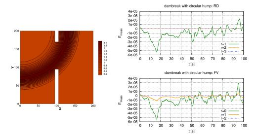
Figure 9: Dambreak with circular hump. Left: bathymetry. Right: dimensionless mass error for different quadrature formula of the bathymetry integral.
