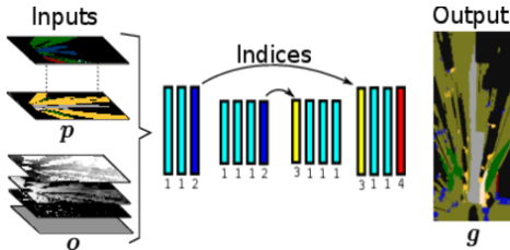
Fig. 4: The fusion network architecture. The number of layers are reduced with respect to a standard VGG16 network. The labels for the layers are as follows: 1: Convolution + Batch Normalization + ReLU, 2: Max-Pooling, 3: Upsampling, 4: Softmax
