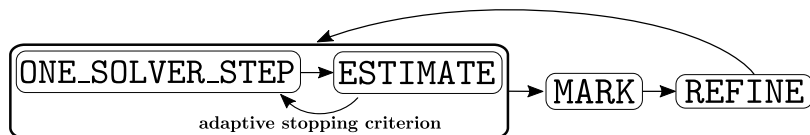
Scheme 2: Paradigm of an adaptive loop employing an inexact algebraic solver.
