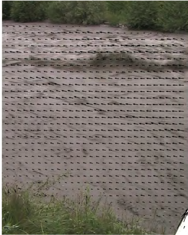
Figure 5.5: Mean dense SGSD velocity field of Arc river second sequence
