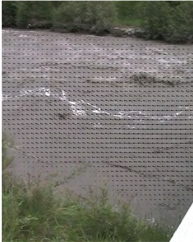
Figure 5.2: Mean dense SGSD velocity field of Arc river first sequence
