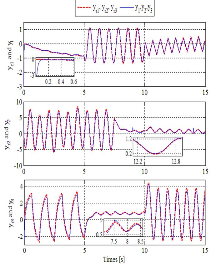
Fig. 2. Outputs trajectory (system and reference model).
