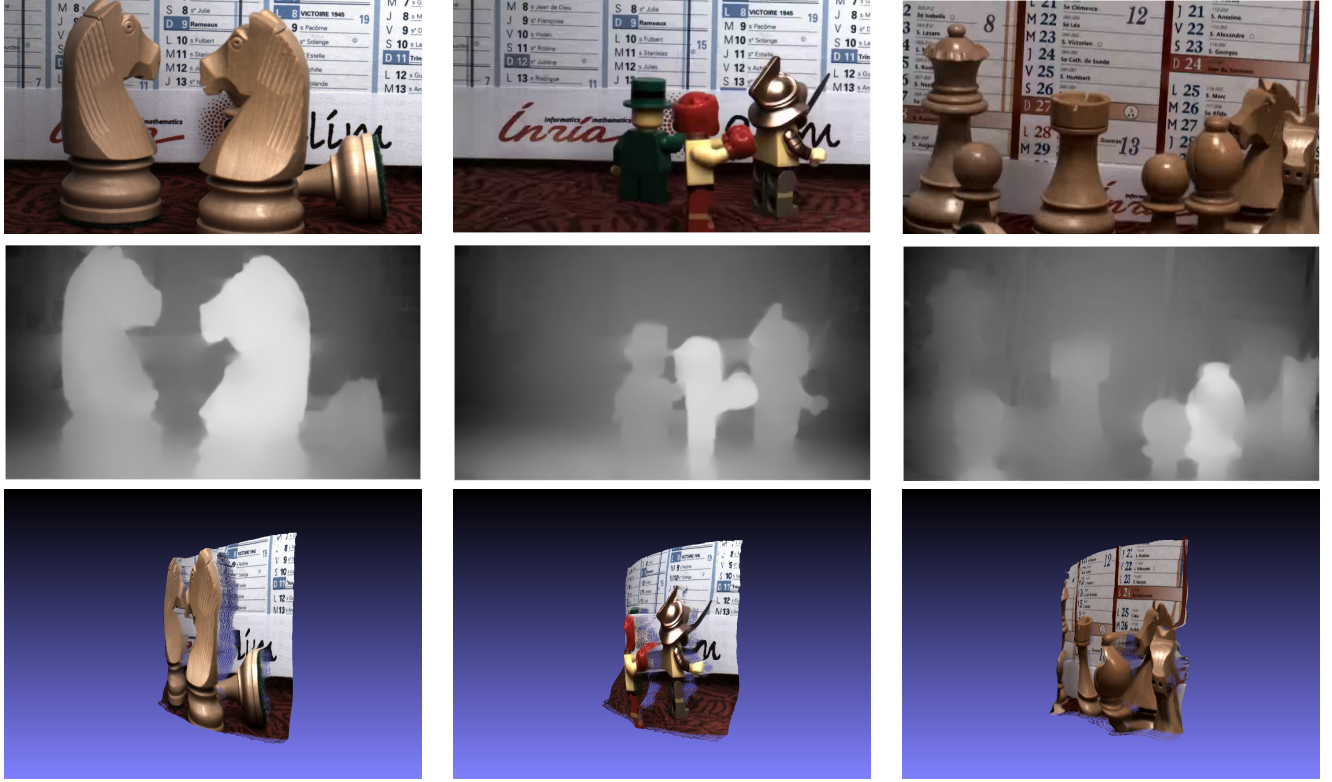
Fig. 2: Examples of the light fields in the new dataset, and the corresponding disparity maps and point clouds: the first row corresponds to the first frame of the central view of each of the three video light fields, the second row to the associated disparity maps, and the third row to the corresponding 3D point clouds, viewed with the MeshLab software program [16].
