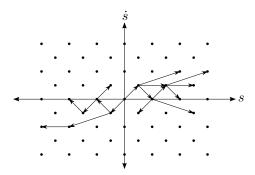
Fig. 3: State space lattice for a 1D double integrator.
