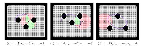
Fig. 11: 2D viability kernel slices of the unstoppable pursuit scenario at different times.
