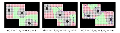
Fig. 13: 2D viability kernel slices of the unstoppable evasion scenario at different times.
