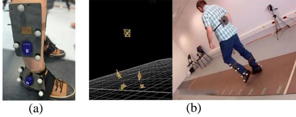
Figure 1. Each subject is equipped with IMUs strapped on rigid support together with 4 reflective markers (a) tracked by an optical motion capture system (Vicon<sup>®</sup>). Subject is instructed to stand still for 5 seconds and then walk five meters on an instrumented walkway mat (Gaitrite<sup>®</sup>), turn at the end of the carpet and walk back to initial position (b).
