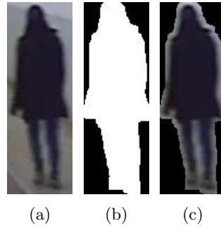
Fig. 8: The multiplication of detected person with its mask, (a) Detected person, (b) Mask of detected person and (c) Results of multiplication
