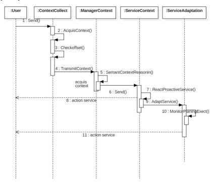
Fig. 3. Sequence diagram for the proactive-reactive framework.
