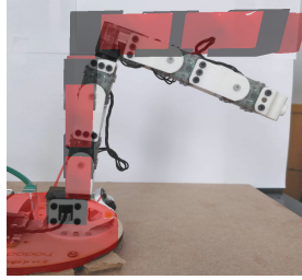
Figure 1: Impact of backlash: when setting both the simulated robot (red) and the real robot (white) to the resting position, the small backlash of each joint adds up to a noticeable difference in the end effector position.
