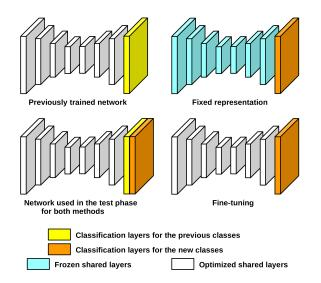
Fig. 5. Example network structures for *fixed representation* and *fine-tuning*. During the test stage, classification layers for the previous classes are appended to the network to generate label maps for all the classes.
