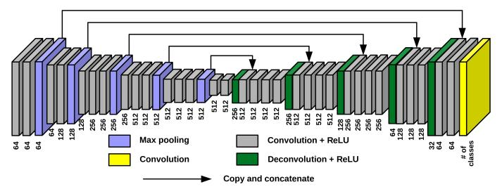
Fig. 2. The network structure. The number below each layer corresponds to number of filters. We refer the last layer, shown by yellow color as the classification, and the rest as the shared layers.
