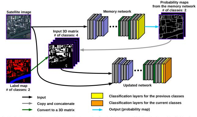
Fig. 3. Adapting the network to the new training data. Although annotations for only 2 classes are provided, the updated network is still able to learn current classes as well as the previously learned 2 classes with the help of the memory network.
