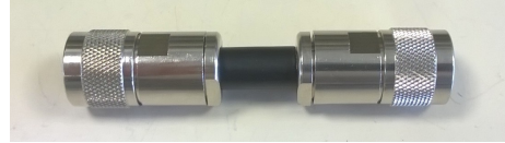
Fig. 1. A pair of connectors mounted on a short cable segment.
