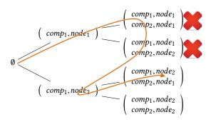
**Figure 3: Search Process Example** (the backtrack search begins by testing to place  $comp_1$  in  $node_1$ , which passes; then it fails to place  $comp_2$  in  $node_1$  and  $node_2$  because of constraint violations; having tested all possible fog nodes for  $comp_2$ , the search backtracks to  $comp_1$  and tries to place it in  $node_2$ . The test passes, and the search continues to place  $comp_2$ ).
