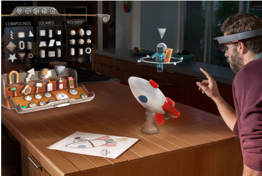
Fig. 1: Microsoft HoloLens is among a new generation of consumer-level Augmented Reality devices that feature interaction through gesture and voice recognition. Courtesy Microsoft - used by permission.
