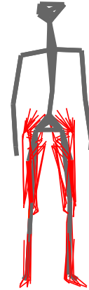
Figure 3. Representation of the musculoskeletal model used in this application. The model exhibits 12 DOF and 82 muscles.
