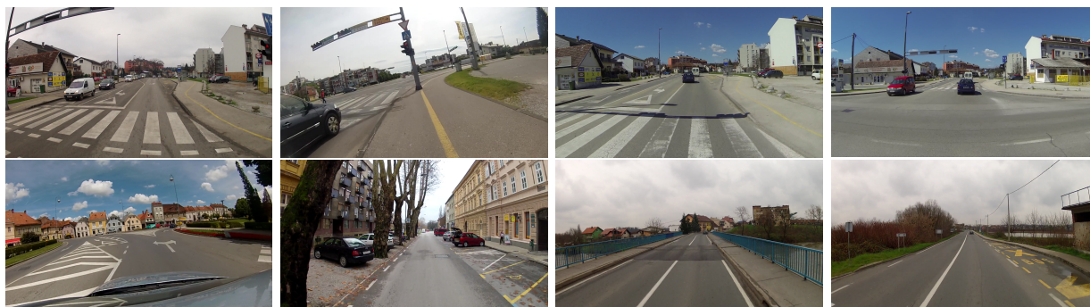
Figure 3: Top row: images extracted for the OSM node with osm.id = 981409265 located at 45.483031 N, 15.546749 E. From left to right: an image in which the zebra crossing was freshly painted, an image acquired from a bicycle, a close-up image in which the crossing was worn-out, and another image from that video taken 20 metres from the crossing. Bottom row: negative images contain many objects with patterns which are similar to zebra crossings.
