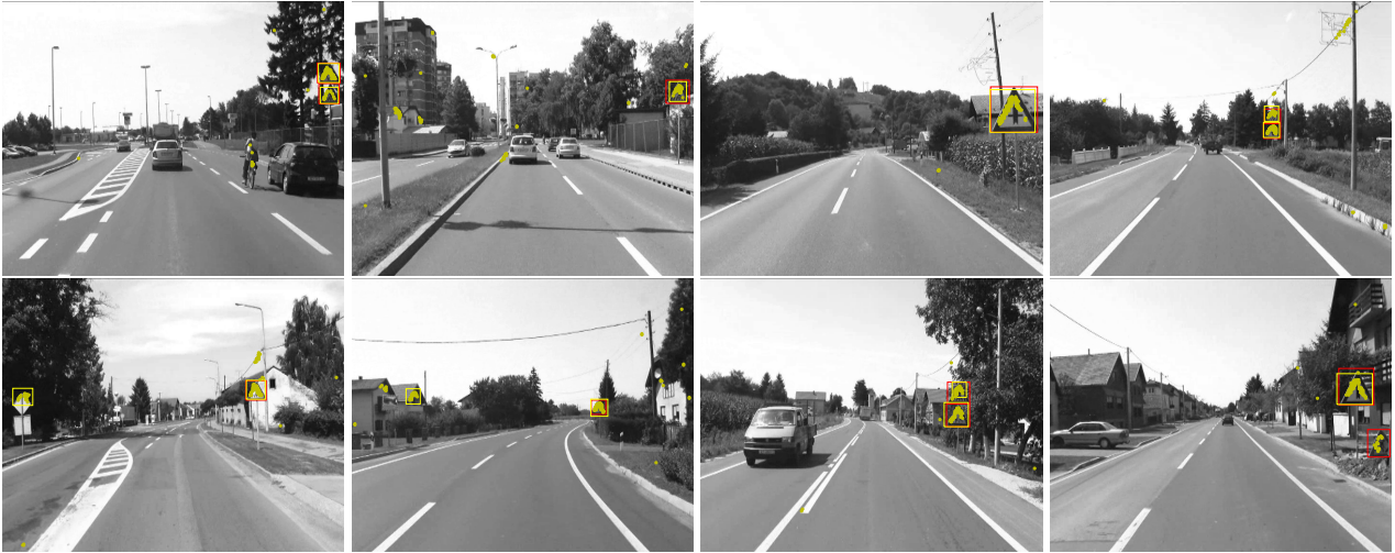
Figure 7: Examples of localization results for traffic signs: the top row shows correct localizations, the bottom one shows examples of failure cases. Localization responses are shown as yellow rectangles, the ground truth annotations (used for evaluation purpose only) are shown as red rectangles, centers of top rated patches are illustrated as yellow dots. The images are shown using grayscale colormap to emphasize the locations of top rated patches.
