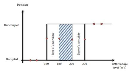
Figure 6: Thresholding circuit and hysteresis in the UM71 receiver
