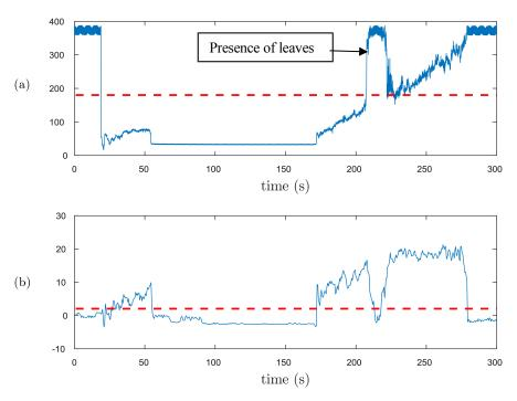
Figure 8: (a) Residual voltage (in mV). The red dashed line represents the threshold of the existing criterion – (b) Criterion of average power in a spectral band centered on the 3OH (in dB). The detection threshold is represented by the red dashed line.
