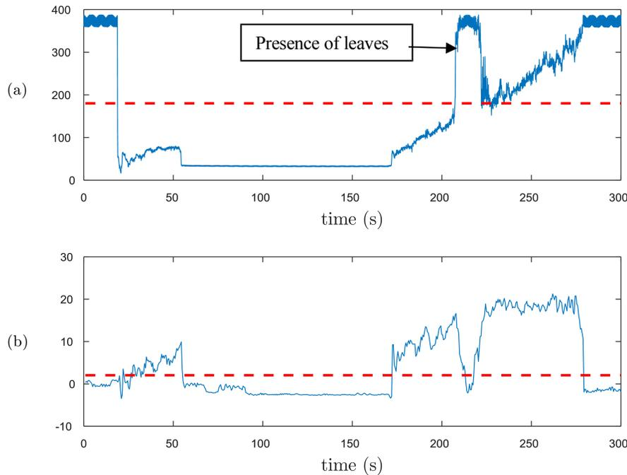
Figure 8: (a) Residual voltage (in  $mV$ ). The red dashed line represents the threshold of the existing criterion – (b) Criterion of average power in a spectral band centered on the 30H (in  $dB$ ). The detection threshold is represented by the red dashed line.
