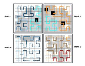
Figure 4: Parallel mesh partitioning using SFC.
