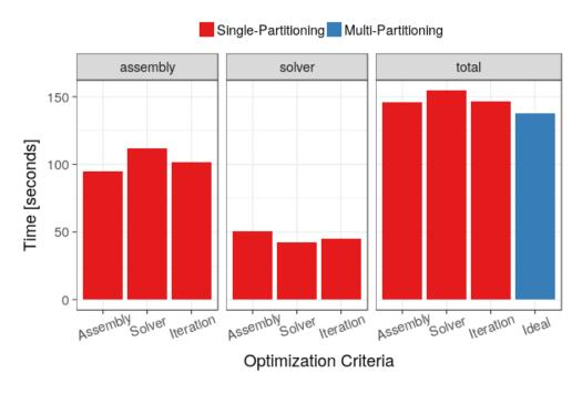
Figure 9: Elapsed time accumulated over a total of 15 time-steps and for the corresponding assembly and solver phases. In blue the estimated total time for and ideal multi-partitioning implementation. Mesh of the respiratory system (28.9M).
