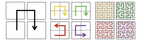
Figure 2: Hilbert SFC parallel generation. a) Initial coarse grid definition, b) orientation of each parallel process to continue the recursion, c) recursive generation of SFC in each parallel process.
