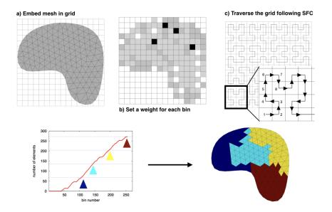
Figure 3: Sequential algorithm for mesh partitioning using the Hilbert SFC. a) Embed mesh in a Cartesian grid, b) Define wights of the grid bins, c) Traverse grid in the SFC order and define subdomains.
