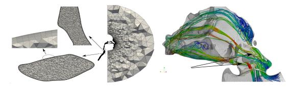
Figure 5: Geometric discretization of the respiratory system (left). Streamlines colored by velocity magnitude and iso-surface of Q-criterion pointing by arrows in the nasal cavities and throat (right).
