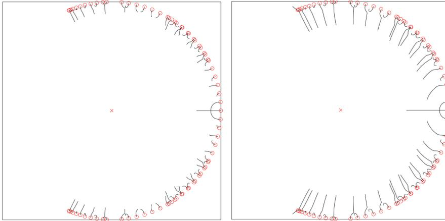
FIGURE 7. Trajectories of the eigenvalues of system (67) in the complex plane (with  $N = 10$  and  $R = R_0$ ). Left:  $\sigma$  varies between 0 and 10. Right:  $\sigma$  varies between 0 and 20. Note that for  $\sigma = 0$  the eigenvalues are all located on the unit circle and their exact location is represented by circles. For  $\sigma \leq 10$  no eigenvalue is of absolute value greater than one. For  $\sigma = 20$  two eigenvalues are of absolute value greater than one .
