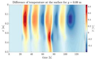
**Fig. 12.** Difference of temperature between pavement with two inclusions and healthy pavement at the surface for y = 9 cm as a function of x position and time. MCP inclusion is located for x between 0.123 and 0.186 m and brine inclusion between 0.311 and 0.375 m
