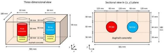
Fig. 2. Schematic view of the domain
