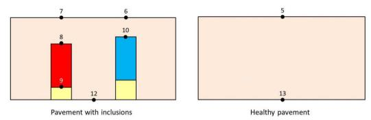
Fig. 8. Sectional view of pavement samples and probes locations with and without inclusion
