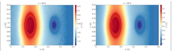
**Fig. 11.** Effects of inclusions on temperature field at the surface at t=25 h. (left: temperature field, right: difference with a healthy pavement)
