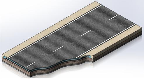
Figure 1: Schematic view of solar hybrid road
