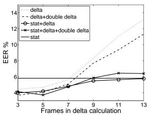
Figure 3. Effect of window size for MFCC delta calculation. Best result is obtained with three frames (equal to STACOG). The baseline system has the same computation pipeline as [12], but with revised MFCC extractor and EER estimation.
