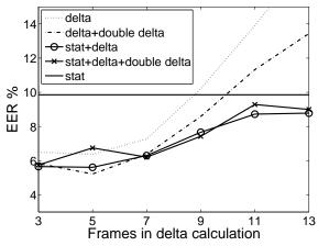
Figure 4. Effect of window size for energy delta calculation. Best result is obtained with five frames.
