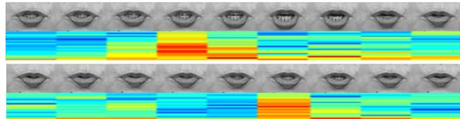
Figure 1. Synchronous lip region frames and audio spectrograms extracted from phrase *Joe took*. Audiovisual synchrony detection seeks to detect discrepancy of the two modalities (an indication of a spoofing attack).
