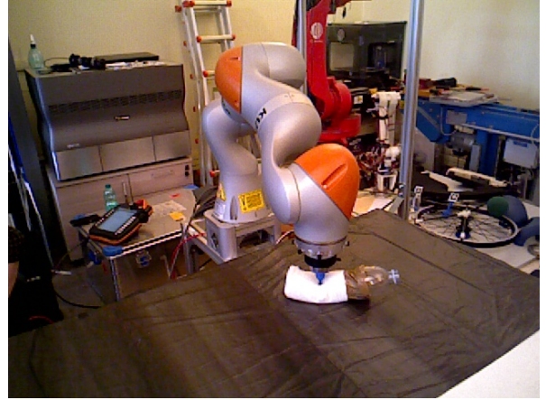
Fig. 1. Setup used for object mechanical parameters estimation.
