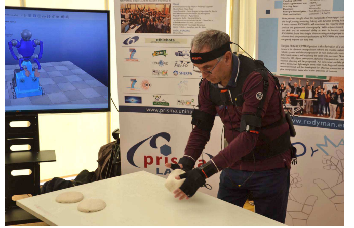
Fig. 7: The renowned pizza chef Enzo Coccia wearing the Xsens MVN suite, with the RODYMAN avatar in the background acquiring and repeating the movements of the chef.
