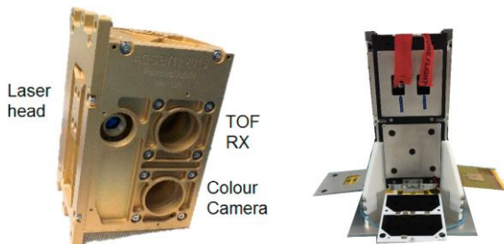
Figure 4. Left: Vision Based Navigation payload, Right: DS-2 target in deployed state
