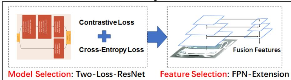
**Fig. 3.** Ensemble methods for image representation: model selection (Two-Loss-ResNet) and feature selection (FPN Extension)
