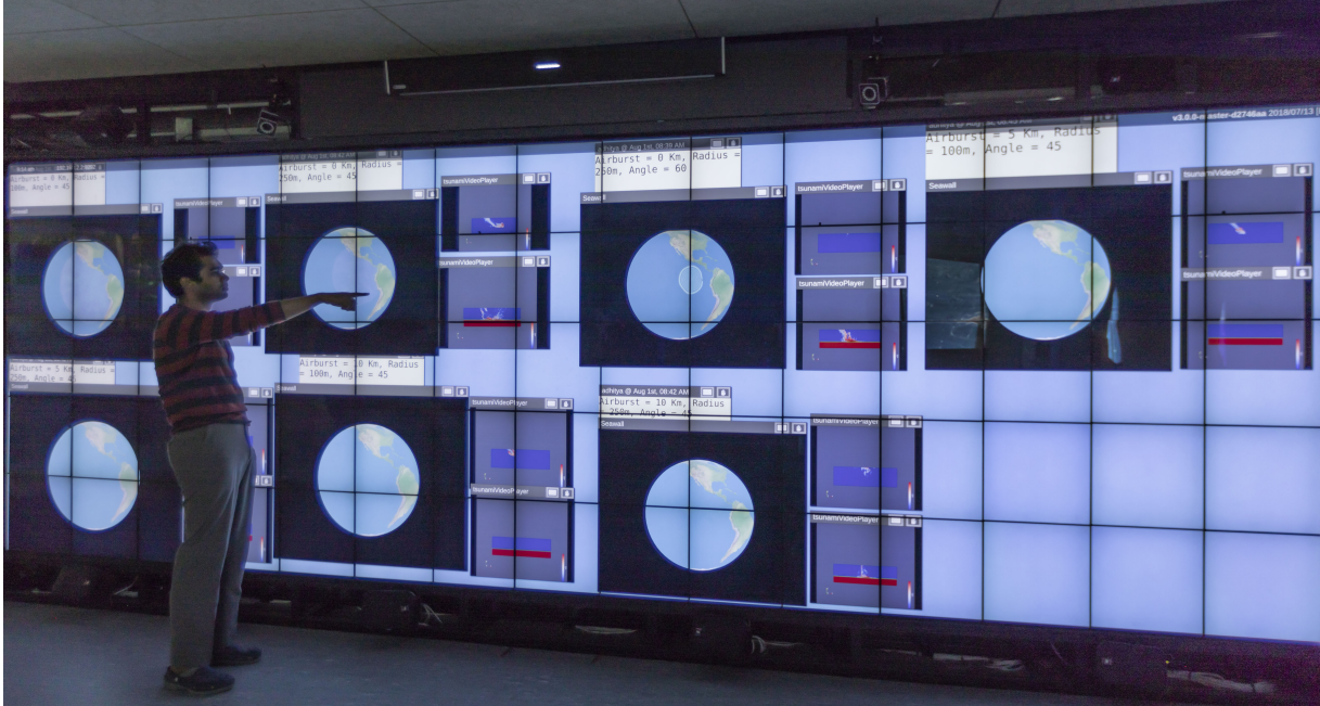
Figure 1: Multiple simulations running simultaneously on the WILDER ultra-wall. The high display capacity of this interactive surface makes it possible to show, for each of the simulations: a planet-wide view showing the propagation of the asteroid-generated tsunami on the globe, a close-up on the region of impact, showing a simulation of one or more scalar fields, parameters of the simulation.
