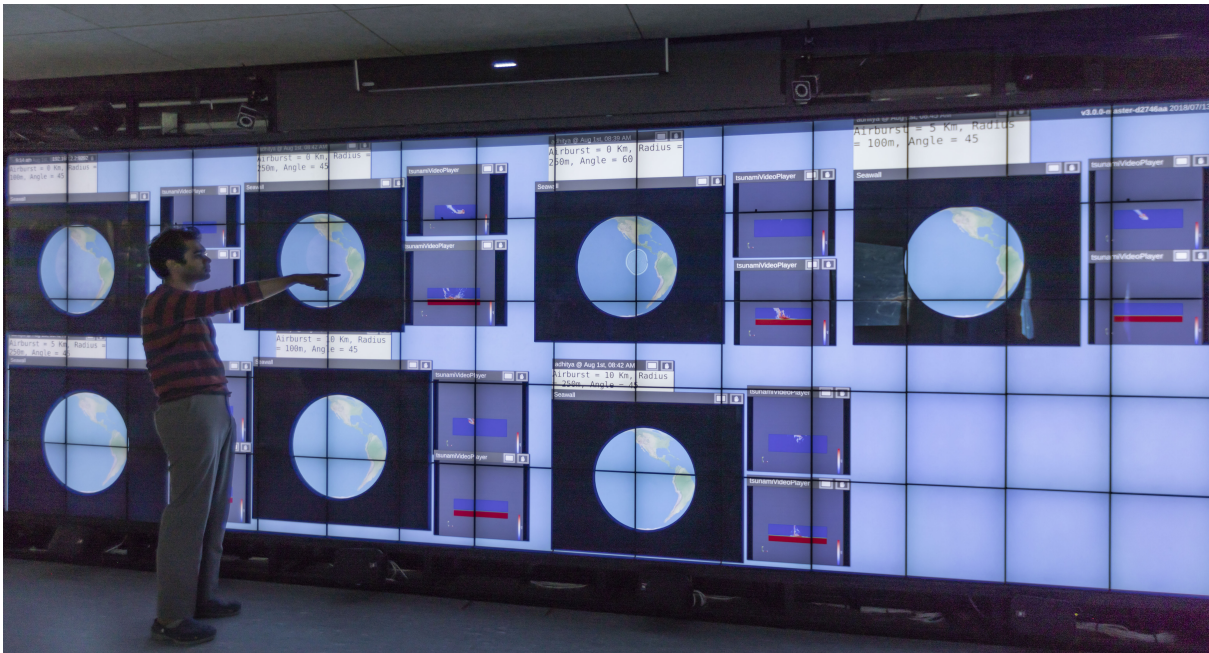
Figure 1: Multiple simulations running simultaneously on the WILDER ultra-wall. The high display capacity of this interactive surface makes it possible to show, for each of the simulations: a planet-wide view showing the propagation of the asteroid-generated tsunami on the globe, a close-up on the region of impact, showing a simulation of one or more scalar fields, parameters of the simulation.
