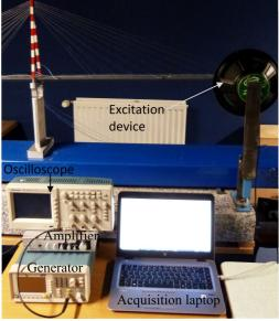
Figure 4. Acquisition and excitation devices
