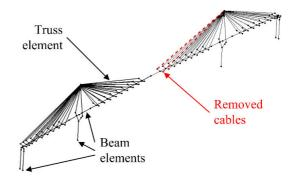
Figure 5. Saint-Nazaire bridge mockup finite element model
