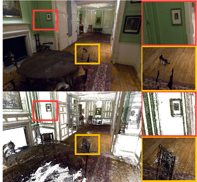
Fig. 4. Top: Globally consistent reconstruction with RealityCapture [2016]. Bottom: Same scene and viewpoint using COLMAP [Schönberger and Frahm 2016; Schönberger et al. 2016]. We can clearly see that the featureless wall is completely missing from the COLMAP depth maps, but a smooth estimate is provided by RealityCapture. Conversely, the details of the back of the chair are only present in the COLMAP depth maps.
