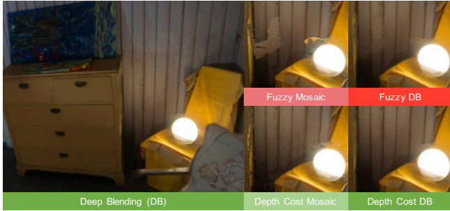
Fig. 9. Our depth cost reduces the effect of “floating geometry” that occurs with a fuzzy depth test [Hedman et al. 2016]. Left: Full view of our output. Middle: Top-ranked mosaic per cost. Right: Network outputs.
