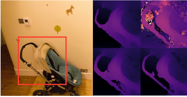
Fig. 5. Merging globally and locally accurate depth maps leads to improved occlusion edge handling and artifact minimization. Left: Reference image Top middle: Globally complete RealityCapture mesh. Top right: Locally accurate COLMAP depth map. Bottom middle: Fused COLMAP and RealityCapture depth maps. Bottom right: Our refined depth map.
