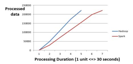
Figure 6 – Performance comparison between Apache Hadoop and Spark Figure 6 itself presents a comparative curve representing the processed data per unit of time between Hadoop and Spark. On this curve, we notice that Hadoop uses 150 seconds to process the 220,000 tweets present in Cassandra (a speed of 1460 Tweets/s), while Spark takes 210 seconds to process the same amount of data. This allows us to say that Hadoop is faster in batch processing than Spark.
