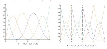
Figure 1. Bézier decomposition (right) from a quadratic B-spline basis (lef) by knot insertion.
