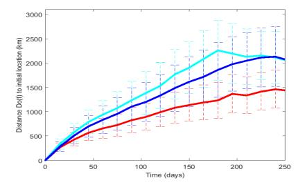
Figure 4. Distance to initial locations of simulated particles barycenter and observed drifter over time, averaged for the 278 drifters found in the tropical Atlantic in the 1992-2008 period. Mean (plain) and standard deviation (dash) are in red for OSCAR-Ichthyop, in blue for ROMS-Ichthyop, and in cyan for observed drifters.
