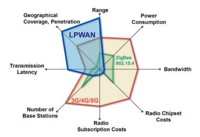
Figure 4. comparative communicating technology of 100 bps.
