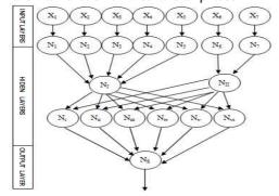
Figure 3. Architecture of the neural network. The variables  $X_1 \, \dots \, X_7$  represent the morphological and frequency properties, respectively the negative form, the maximum amplitude, the minimum amplitude, the maximum width, the minimum width, the hearth rate and the hearthbeat. The variables  $N_1$  ..  $N_{vi}$  represent the intermediate nodes. The Node  $N_s$ determines the arrhythmia type.
