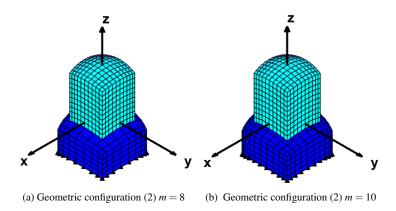
Fig. 20: Configuration (2) example of inconsistent meshes
