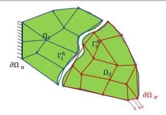
Fig. 6: Inconsistent mesh partition that introduces geometric inconsistency:  $\Gamma_1^h \neq \Gamma_2^h$ , second case curbed interface
