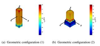
Fig. 17: Von Mises stress under pure traction load case
