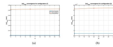
Fig. 25: Convergence of the maximum displacement with mesh density: (a) for configuration (1) and (b) for configuration (2). The mesh was changed keeping the same element aspect ratio and the conforming interfaces in figure 13under the form  $n \times n \times 10$  for the upper domain of configuration 1 and  $m \times m \times 10$  for the upper domain of configuration 2
