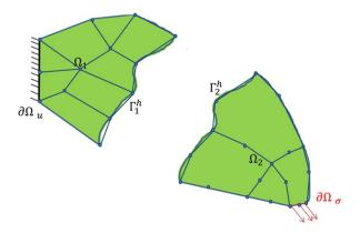
Fig. 7: Inconsistent mesh partition that introduces geometric inconsistency:  $\Gamma_1^h \not\equiv \Gamma_2^h$ , third case different shape functions
