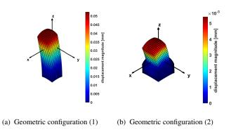
Fig. 16: Displacement amplitude under bending-traction load case
