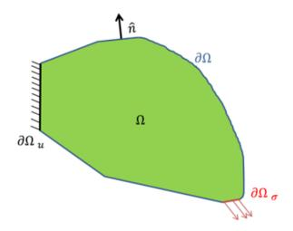
Fig. 1: linear elastostatics problem definition
