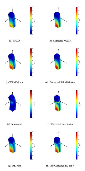
Fig. 23: Von Mises stress plot configuration (1) under bending-traction load case, for n=4 and  $\Gamma_2$  master.
