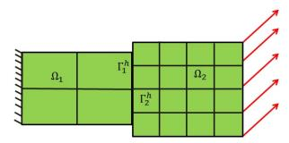
Fig. 5: Inconsistent mesh partition that introduces geometric inconsistency:  $\Gamma_1^h \not\equiv \Gamma_2^h$ , first case different mesh boundaries
