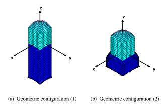
Fig. 13: Geometric configurations (1) and (2), pure traction load case
