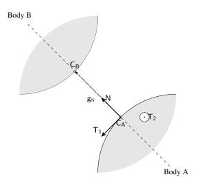
Fig. 1: Contact kinematic
