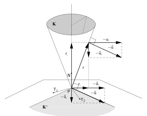
Fig. 2: Coulomb's friction law in the sliding case.
