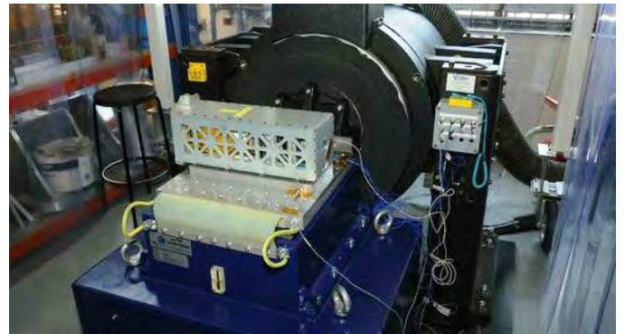
Fig. 35: Dragsail: Vibration EVT Testing. With EQM unit.
