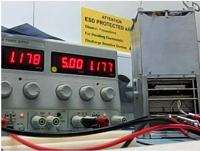
Fig. 9: DS-1: Burnwire Testing.
