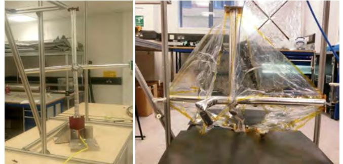
Fig. 11: DS-1: Inflatable Functional Testing. Left: inflation testing from SQM without sail segments. Right: inflation testing from SQM with sail segments attached (mid-inflation). Both tests using external gas supply line.
