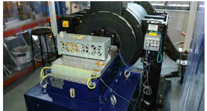
Fig. 35: Dragsail: Vibration EVT Testing. With EQM unit.
