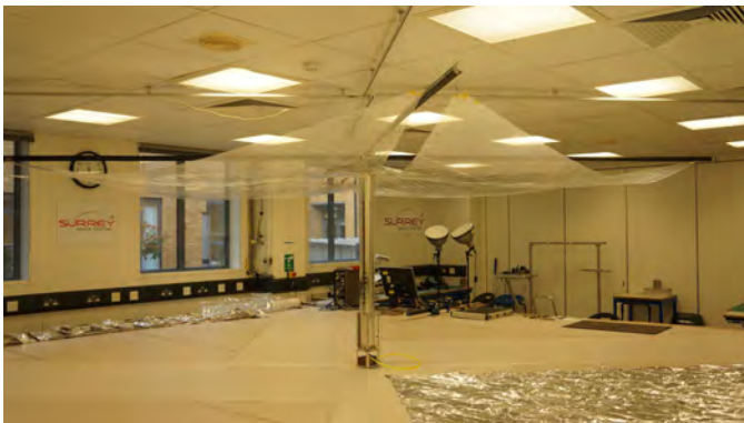
Fig. 33: Dragsail: Deployment Test. With EQM unit.
