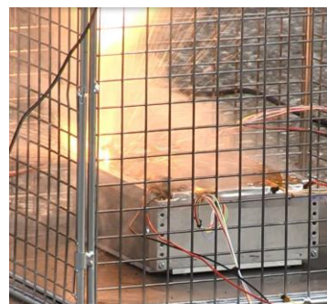
Figure 13. Test Battery induced into thermal runaway
