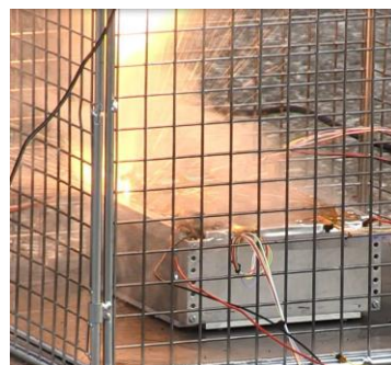
Figure 13. Test Battery induced into thermal runaway
